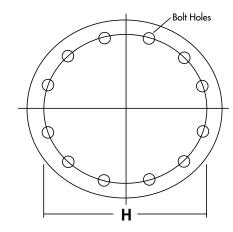
H= Center to Center dimension of Opposite Bolt Holes (Bolt Circle Diameter). If this dimension cannot be measured, find center to center of adjacent Bolt Holes
